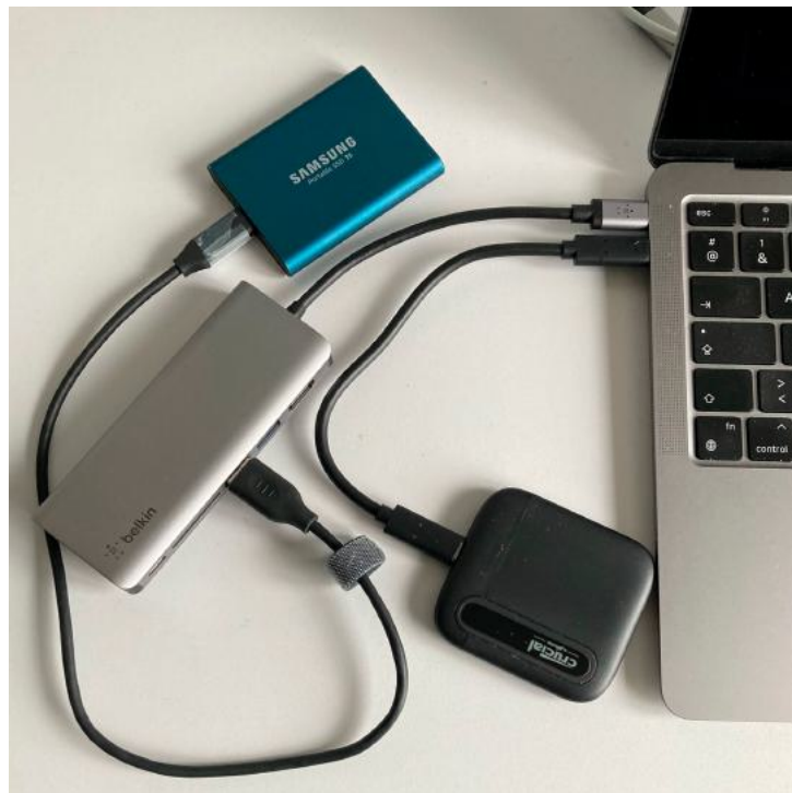
T7 drive connected via a hub and Crucial SSD connected to a MacBook port.
