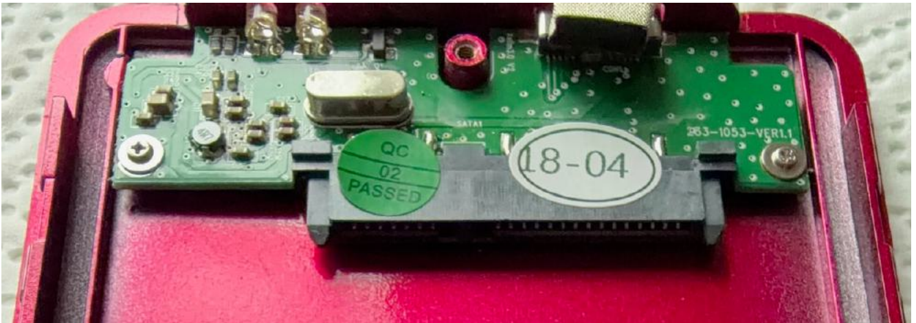
Close-up of the connector for the drive to be inserted (SSD or HDD).
