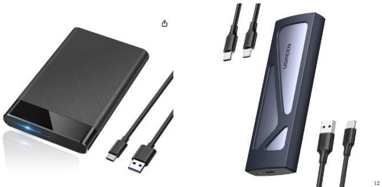
On the left, an enclosure for an SSD; on the right, an enclosure for an NVMe drive.
